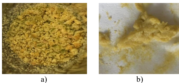
Picture 1. a) Dried and shredded mandarin peels b) Pectin obtained by boiling in an acidic medium, dissolving in ethanol, and filtering through filter paper.
